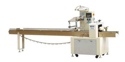
The horizontal flow wrapping machine is also named as Pillow Packing Machine comprises of transmission rack and sealing Equipment. The flow wrapper is good for OPP/CPP PT/PE, KOP/CPP, ALU-FOIL packing material.
