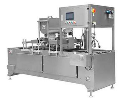
YFS-6 is a filler/sealer produced and designed for medium/large productions. It is perfect for high precision packaging, sealing and checking up to 4000 pieces per hour.
