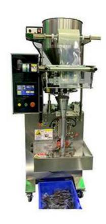
This bag filling sealing machine is mainly used to pack liquid, cream products: such as shampoo, cream, oil, honey, sauce, etc. It can finish bag making, filling, 3/4 side seal, coding in one machine.
