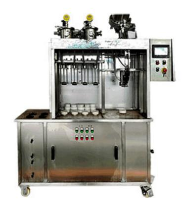
Four heads semiautomatic beer bottle rinsing, filling, capping triblock machine main parts are automatic electronic control filling valve, vacuum preparation of pressure (CO2), the photoelectric liquid level detection automatic filling process, CIP cleaning system, bottle deformation pieces easy-worn parts.
