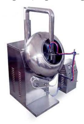
BYC-600 Sugar coating pan, sugar coating machine. This sugar coating machine manufacturer is used to carry out sugarcoating and film coating to the core of Chinese Traditional and Western Medicine tablets; it integrates strong power, weak power, hydraulic and pneumatic. It is new type equipment...
