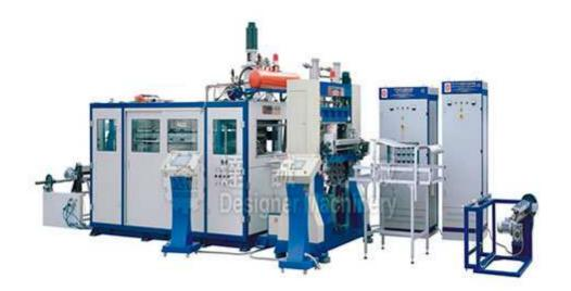
Our company is a professional continuous thermoforming machine with punching machine supplier in China. This kind of automatic thermoforming machine with punching cutting stacking is controlled by servo, which can produce all kinds of packaging sheets with PP, PET, PS, HIPS, PVE and other plastic materials. The machine has three stations that include forming, cutting and stacking station.
