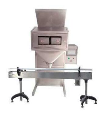
The FF-C02A digital control particle filling machine is suitable for packaging materials with good fluidity such as washing powder, dry seasoning, seed, salt, feed, mono sodium glutamate, white sugar and so on. The digital control particle filling machine can weigh and fill the powder and particle into preformed bags, bottle, cans etc.. It can fill materials from 100g to 2500g according to the materials. It is suitable for flour, milk powder, chili powder, bean, peanut, nuts etc.
