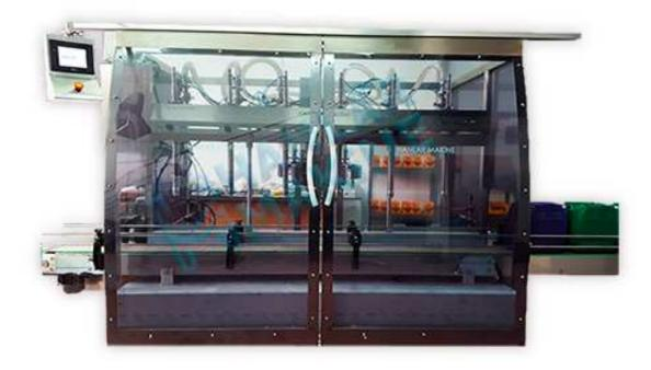
BT 500 Canisters Cans filling machine. Filling system Load Cell or Flowmeter is filling 5-40kg filling range, easy cleaning, and simple design high filling accuracy.
