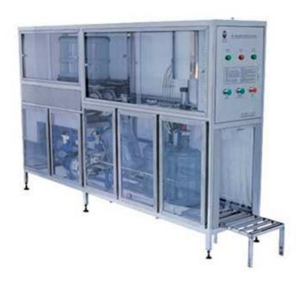
The whole process of bottle washing, filling and sealing is produced in the closed channel, which can effectively prevent pollution and ensure the sterile and pure water quality.
