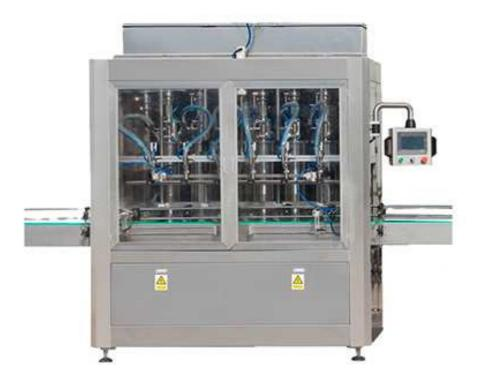
This machine used to filling 500ml-5L PET bottle food oil, cooking oil. Also it can use to filling bottle water, juice. beverage, drink, which the bottles don't neet to washing/rinsing.
