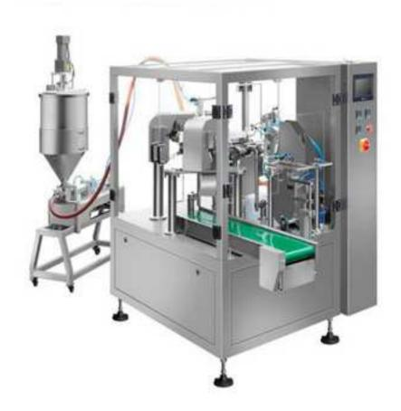
This set of equipment is made up of bag feeding packaging machine and paste filling machine. It is mainly used for automatic measurement packaging of liquid paste materials such as washing liquid and fruit juice.
