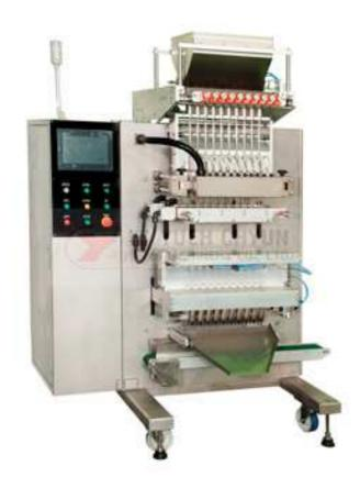
The multi-lane auto filling sealing packing machine is up to 10 lanes of stick packages, it is widely used for sugar sticks, coffee creamer sticks or coffee powder sticks and so on.
