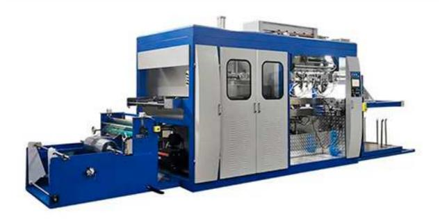
Vacuum forming, also known as thermoforming, vacuum pressure forming or vacuum molding, is a procedure in which a sheet of heated plastic material is shaped a certain way.
