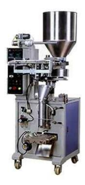
The Automatic Stick Granule Packing Machine is suitable for packaging non-sticky, bulk or granular materials, such as medical pills, food, plant seeds, washing powder, coffee, sugar, desiccant and so on.
