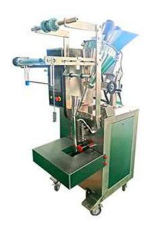
This machine is equipped with a dual-CPU microcomputer control system, a 5-inch LCD display in Chinese or English, a humanized operation interface, automatic cursor detection and tracking, and simpler operation. Equipped with a high-precision stepping motor to ensure the accuracy of the cutting position of each packaging bag.
