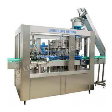
Glass Bottled Sparkling Water Filling Machine Is Designed On Counter Pressure Filling. The Cap Could Be Crown Cap, Screw ROPP Cap, Pull-Ring Cap, Or Twist Off Cap. Speed Is From 2000bph To 18000bph. Bottle Washing At the First Step, Then Bottle Filling And Capping. After Bottle Capping, Filled Bottles Be Transfered to Labeling Machine, Packing Machine.
