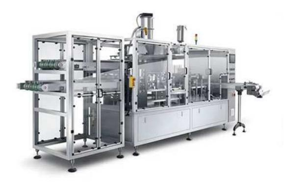
CE Approved professional Nespresso coffee capsule filling machine is suitable for filling and sealing Nespresso, k-cup, lavazza, dolce gusto and caffitaly all kind of coffee capsule. It is widely used to coffee powder milk powder, tea powder etc. The speed can be 80-220 pcs per min. and also can be easily to depend on customer requirements to change machine.
