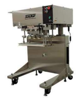
The semi-automatic, straight line, six spindle SK600 Cap Tightener & Retorquer can handle all standard cap torquing duties. It tightens pumps and trigger sprayers where automatic insertion of the pumps and triggers is not feasible. This model is useful after induction sealers to ensure caps are properly retorqued before leaving the line. It can be upgraded to a fully automatic capper.
