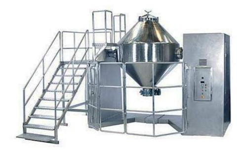
**PMS DOUBLE MIXER®** is a tumbling mixer suitable for gentle blending of dense powder and granules. It has been recognized as an economical tumbler with its durability and minimum maintenance requirement. Our product series range from 150 to 1,600 liter in working volume.
