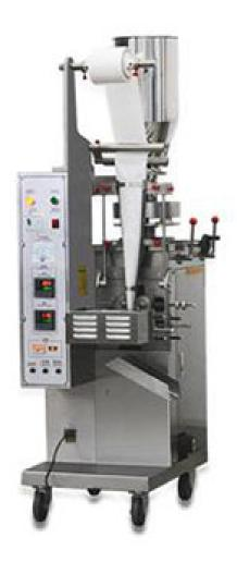
The MK-T10 vertical form fill seal machine is intended for packaging products like tea and coffee. This tea bag packaging machine produced tea bag has a cotton string. The tea bag is formed at one time to avoid direct contact between hands and materials, more sanitary while improving packaging efficiency. Mingke pack can help clients to meet their requirements for perfect packaging by adjusting the bag size and fill product weight slightly.
