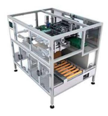
The automatic packing production line is mainly composed of pusher parts, tray parts, conveying parts, frame parts, pneumatic parts and direct parts, which can complete automatic feeding of rolls, automatic arrangement of rolls, automatic loading of rolls.
