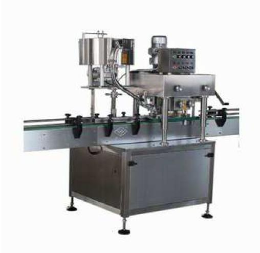
This capping machine is mainly used for locking caps for bottles of daily chemicals, medicine, chemical industry, such as nozzle, pump head, spray pump and hand button spray gun and so on.
