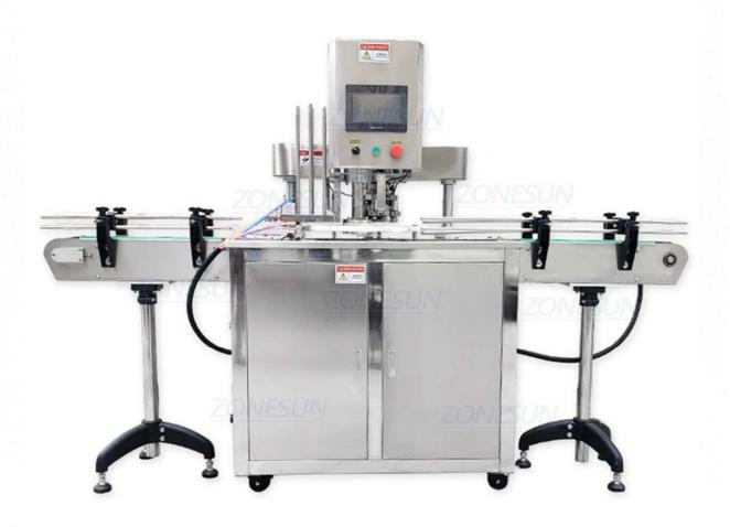
Suitable for all kinds of iron, plastic, aluminum cans and caps, glass, paper cans. For the capping of the tinplate cover, aluminum cover.
