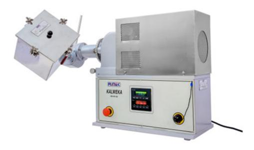
Cube Mixer is based on a movement, which through its tumbling effect produces a homogeneous mixture in the shortest possible time. The product to be mixed is treated very gently. The cube mixer can be attached to the universal gear (UD). The mixing movement of the product in the mixer is deflected and interfered with by 3 mixing rods made of stainless steel.
