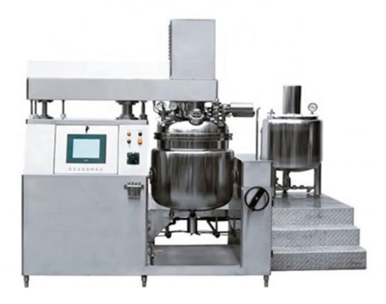
The whole equipment of this system is composed of emulsification mixing tank, boiler, pretreatment boiler, vacuum system, hydraulic system, electric control system, material discharging system and working platform.
