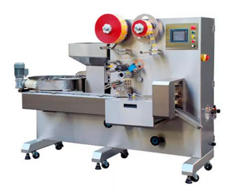
The candy wrapper for hard candy pillow type packaging can be equipped with 1 servo or 3 servo driven for different production capacity requirement. Flow pack machine for hard candy
