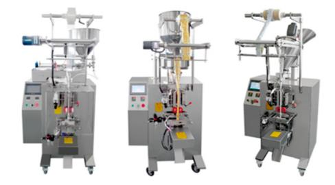
Optimized design, stable performance and simple operation; Strong expansion function, can add bag connecting device and inflation device. Meet the needs of different products; The product structure is reasonable and convenient for cleaning and washing; Bag making, measuring, filling, sealing, printing date and product output are completed at one time.
