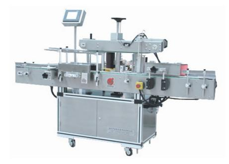
The machine is especially designed aiming at the industry of daily chemical products, medicine and foodstuff. It is used in many symmetry or inappropriate round/flat/square vessels label-sticking in all around. Simple adjustment and wide applicability: Having a little adjustment, it can change each other between rolling sticking and side sticking. One machine can complete multi-size vessels label-sticking (round/flat/square bottle).
