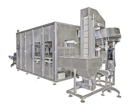
TGJ-1 Cap Applicator used for pasting cap on the packages. Rotary disk sorting mechanism, glue and cap feeding system adopt cam and servo drive system, continuous, high-speed paste.
