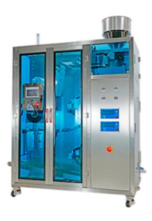
This Drip coffee Bag Packing Machine is engineered to precisely fill and seal hanging ear coffee bags, ensuring consistent quality and freshness. Its user-friendly interface allows for easy operation and customization of packaging parameters. Designed for efficiency, it boasts high-speed packing capabilities while maintaining accuracy and reducing waste. Ideal for small to large-scale operations, this machine enhances productivity and ensures a professional presentation of your coffee.
