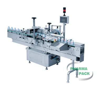
The label strip from the label roll holder is spread around several guiding rollers, through the dispenser and fixed on the base paper recycle roller lastly. Bottles are fed via the spacing wheel. When the sensor detects the coming bottle, it will signal the label dispenser to stick out a piece of label, which is stripped off by the passing bottle. Then the label will be pressed closely against the bottle surface by the label wrapping device.
