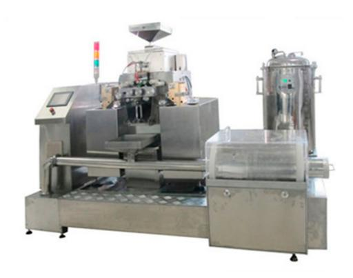
HTSYS-5 soft capsule machine is my company in 2010, the latest development of new products, the machine is only the smallest model laboratory soft capsule machine, carefully designed in full accordance with GMP requirements. The single-phase 220V power supply, mainly used in soft capsule product development laboratories and drug research institutions and colleges teaching demo.
