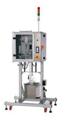
Tamper Evident Band Applicator, CH-100 is designed with SUS frame to match production requirement of Foods & Pharmaceutical industries. Modularized machine body & assemblies for quick adjustment & parts change. Cutting Unit is designed with quick change feature to save changing time of cutting blade. Also, machine could be installed remote control feature to monitor production.
