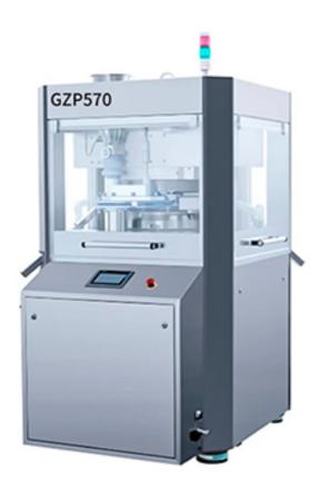
This machine is one kind of double side rotary tablet press machine, which can press granular materials into round shape tablet, irregular tablet or double-side engraved tablet. This machine is mainly used in pharmaceutical, chemistry, foodstuff, electronic industries.
