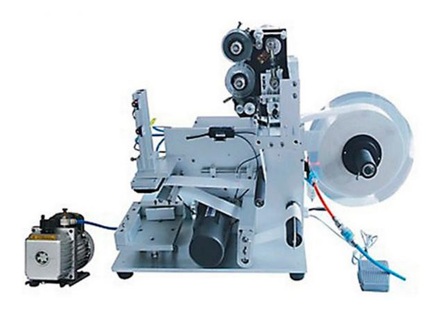
Imported high-precision intelligent electric eye and high-reliability computer chip program controller (PLC) are used to control the labeling. The air pressure is used to adsorb the self-adhesive label on the label head, and the labeling head cylinder is used for labeling.
