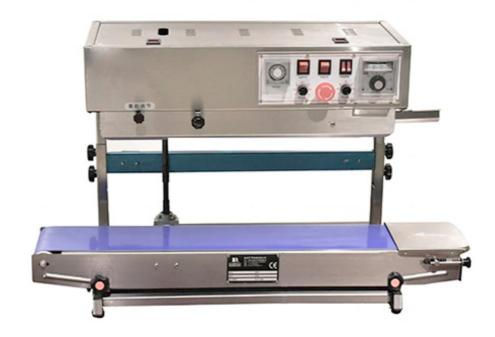
This series multi-functional film sealer (with solid inker printer) is suitable for small bags packaging and adopts electronic constant temperature control system and speed adjusting transmission mechanism. It can seal plastic films of various materials. Such as PE, PP, Aluminum foil. And can be fixed date embossing system.
