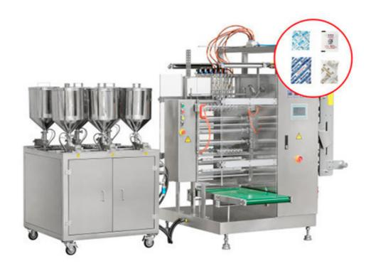
The DC-880(L/G) multi-row high-speed packaging machine is suitable for packaging equipment for materials such as liquids, viscous substances, or granules.
