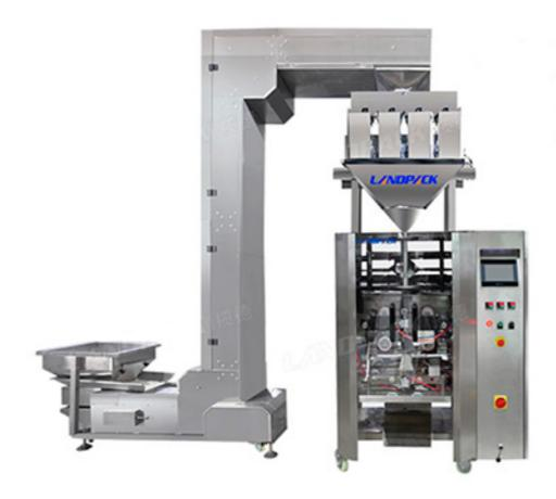
This packing machine is suitable for weighing and packaging various granular products and powder products, such as oatmeal, sugar, salt, seeds, rice, sesame, washing powder, detergent powder packing machine, puffed food, casserole, candy, potato chips, nuts, frozen food, small hardware, medicinal materials, etc.
