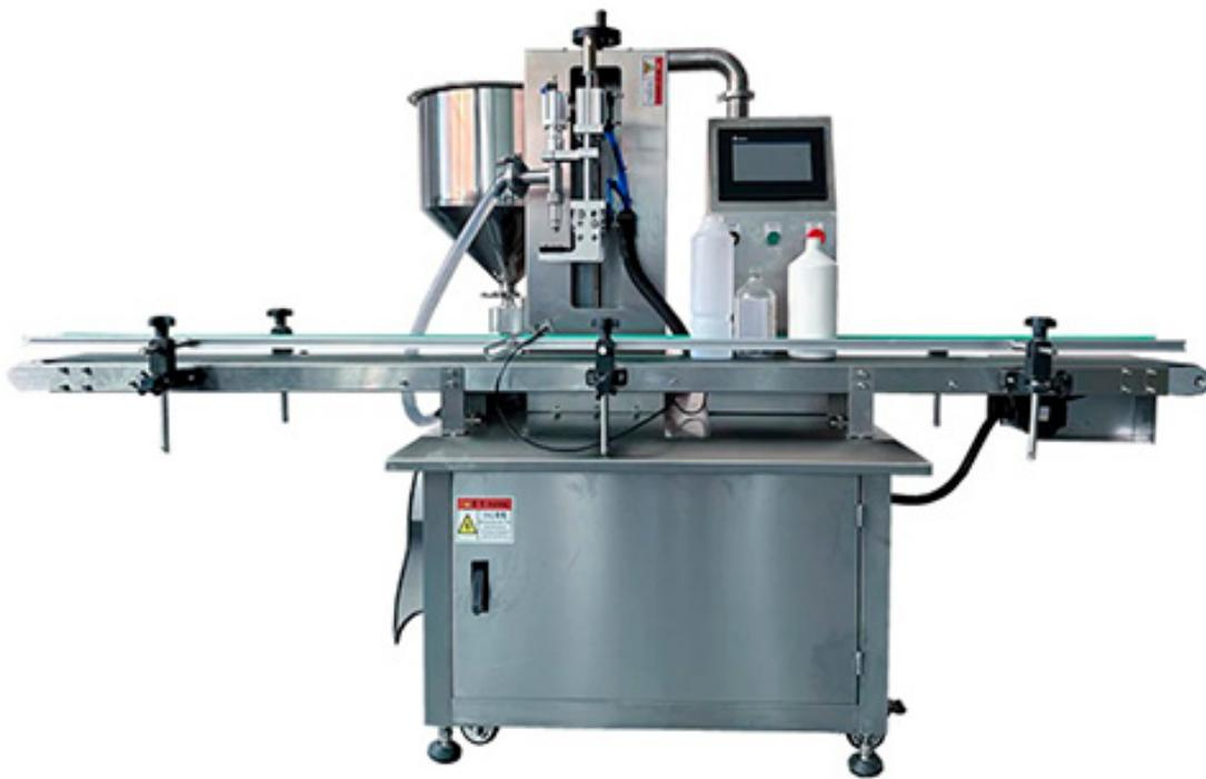
The automatic single-head servo gear pump filling machine is a high-precision and efficient filling device widely used in industries such as cosmetics, pharmaceuticals, food, and chemicals. It is designed for the accurate dosing of liquids, viscous fluids, or semi-fluids. The machine uses a servo motor-driven gear pump to ensure a stable and precise filling process. Below is a description of its main features:
