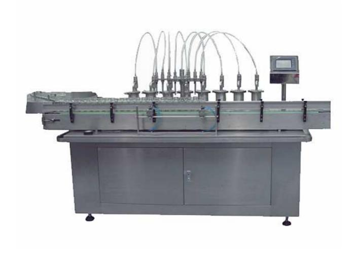
This machine is the main filling equipment of liquid filling production line, which is mainly applied in the filling of 50 - 500 ml glass bottle or plastic bottle. Equipped 6 to 16 filling nozzles, precise filling, and no bubble. Advanced design, compact structure.
