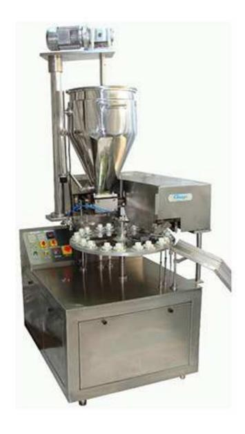
'GMP's' Semi Tub Filling & Sealing Machine work on volumetric principle The unit is made compact, versatile and enclosed in stainless steel elegantly matt finish body, Reciprocating Nozzle with self-centering devices & SS Syringe. No tube No filling system arrangement is standard features of the machine.
