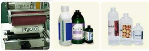
Suitable for wrap-around labeling on round bottles in small quantity and with high labeling precision and quality requirements. Also able to handle bottles with orientation requirements. Manual placement of bottle. Easy operation. High quality output.
