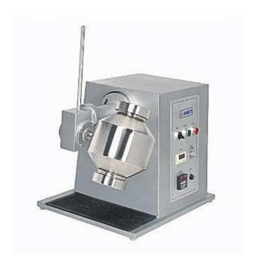
Double cone operates on free flow principle. This unit is used for rapid mixing of all types of free flowing powders and granules. The uniform, multidimensional arrangement of the mixer walls ensures good mixing. The vessel is manufactured from stainless steel and secured with threaded Cap. This unit can be attached to the Universal Gearing.
