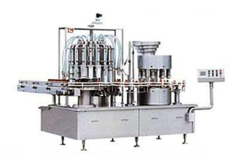
**Usage:** feeding bottle, air blow and vacuum sucking to clean bottle, high speed rotary filling liquid (syrup) in bottle, feeding cap and screw capping.
