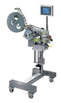
Automatic label applicators are useful when higher volumes and Labeling on conveyor lines are needed. A sensor detects the product as it comes down the conveyor and triggers the application of the label at the proper time. Product handling must be tightly controlled to ensure accurate label placement.
