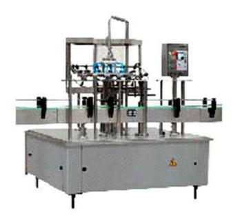
The machine reference to co generic Product's Technology and design principle in abroad, High efficiency in flushing bottle, Adopt continuation water following flushing way bottles automatic overturn. Applicable to the new bottles of flushing and drain, Automatic operate from bottle in until bottle out, Blunt ozone disinfectant Equipped with a sterile compressed air ventilation device, it's the Ideal cleaning equipment for wine cosmetic medicine and food industry.
