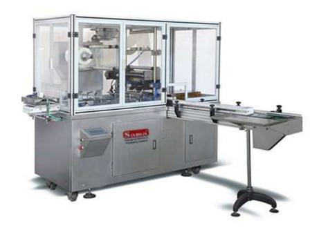
Overwrapping machine is used to wrap the products. For instance; cigarette boxes overwrapping machine, mobile phones overwrapping machine, boxes overwrapping machine, candy boxes overwrapping machine, perfumes boxes overwrapping machine and all those products that are packed in boxes or cartons.
