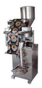
Granule Packing Machine is suitable for pharmacy, food, household chemicals, plastic products and other special industry and other loose type and in viscid granule material. Such as seeds, Chinese Drugs, feeding stuff, medicinal granules, pillar, monosodium glutamate, salt, sugar, soup blend, oat, tea, active carbon, washing powder, dryer, etc.
