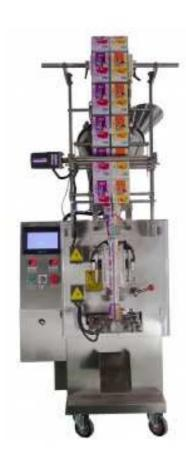
This machine is applicable for powder packaging used for packing powder in field of food, medicine and chemical.
