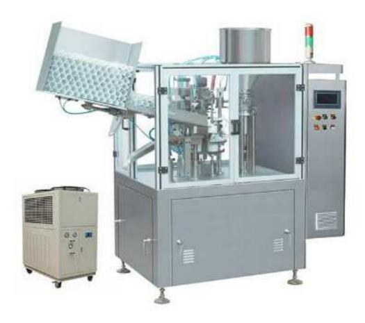
Plastic Tube Sealing Machine widely used in pharmaceutical, food, cosmetic and daily chemical industries to fill ointment or viscous fluid materials into plastic tube or laminated tube. And then seal the tube tails irregularly trim the tails and print batch number & production date on tubes.
